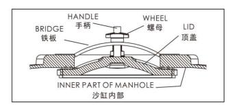
Introduce the lid in the manhole, leaving it leveled and centered. The lid must be supported by the handle, as this will avoid that it could fall into the tank and damage any of its parts. Put the bridge in the position shown and tighten manually the wheel. To achieve a proper seal, you do not have to tighten excessively the wheel, as this could damage the lid. The pressure itself will improve the seal.
